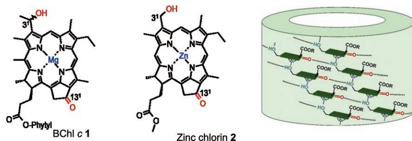
Scheme 1. Structures of naturally occurring bacteriochlorophyll c 1 and zinc chlorin model compound 2 , and a model showing the three noncovalent interactions involved in the formation of supramolecular rod aggregates (right).
